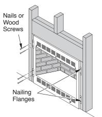
Figure 23 - Attaching Firebox to Wall Studs
